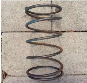
**Gambar 2 Pegas CVT 800 Rpm (standard)**
